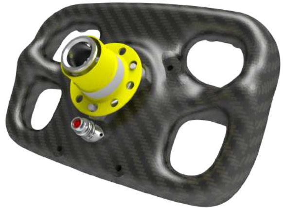
Steering wheel's CAD (rear part).
