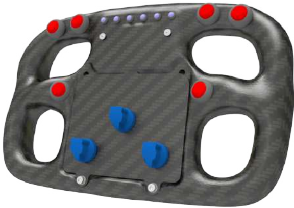
Steering wheel's CAD (front part).
