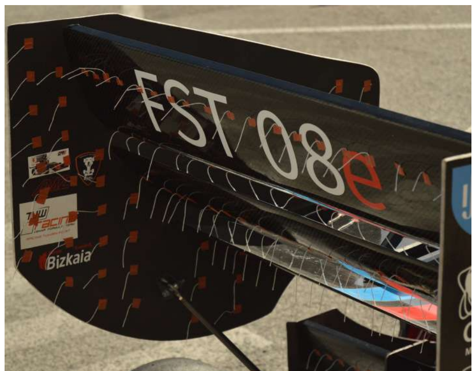
Detail of the small threads of wool in the rear wing.
