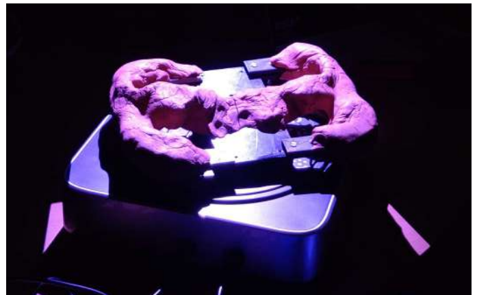
Scan to the steering wheel's handles.
